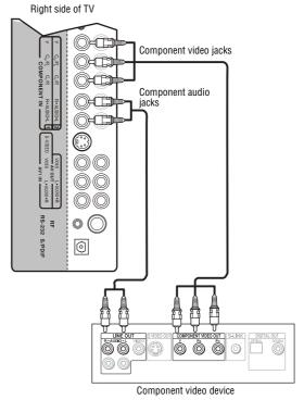
3 Connect an audio cable to the COMPONENT 1 AUDIO or COMPONENT 2 AUDIO jacks on the right side of your TV.
